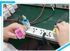
9. Aging test for travel charger
